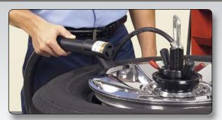
Directs burst of compressed air to easily seat the bead
