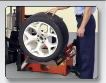
Optional wheel lift eases servicing of large assemblies. Allows for careful handling of expensive wheels. (20-2517-1)
